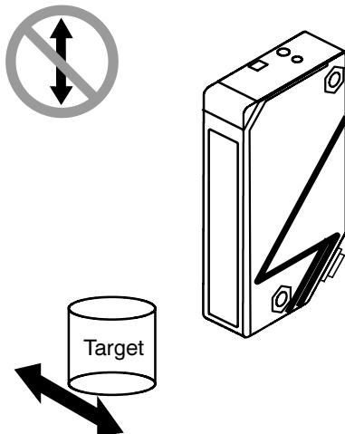
**Note:** Due to the detection method, targets traveling horizontally to the sensor's optics are detected. Targets traveling vertically may not be accurately detected. For reliable background suppression, a minimum separation distance of 6 mm is recommended between the target and the background.
